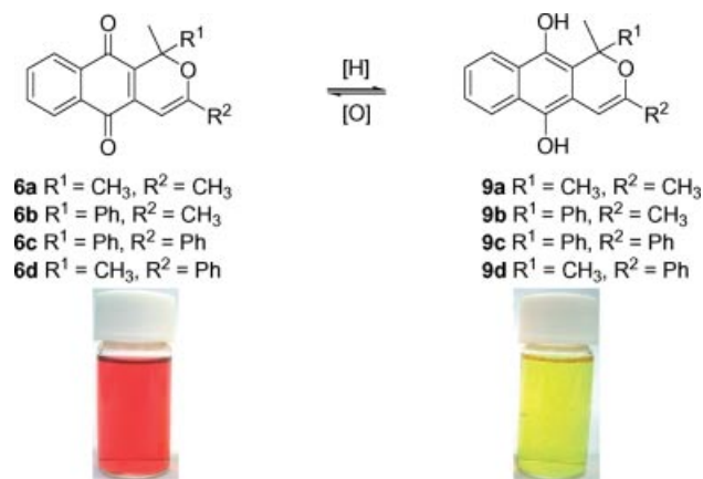
Figure 3. The redox switch between 6a–d and 9a–d , and the corresponding colors in the oxidized (left) and reduced forms (right).
